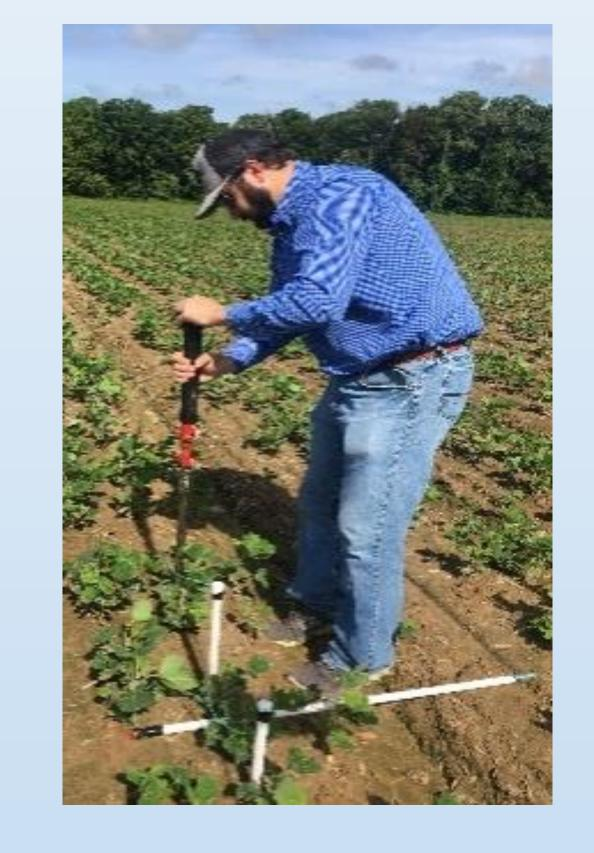
Local producer, Alex Kehrees installing watermark moisture sensors in field in Phillips County
