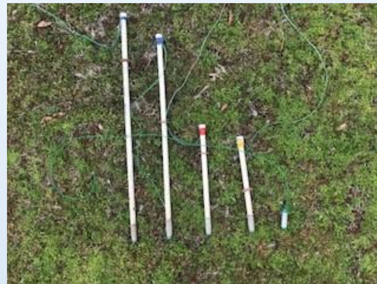
Moisture sensors before installation L-R 30" to 6"
