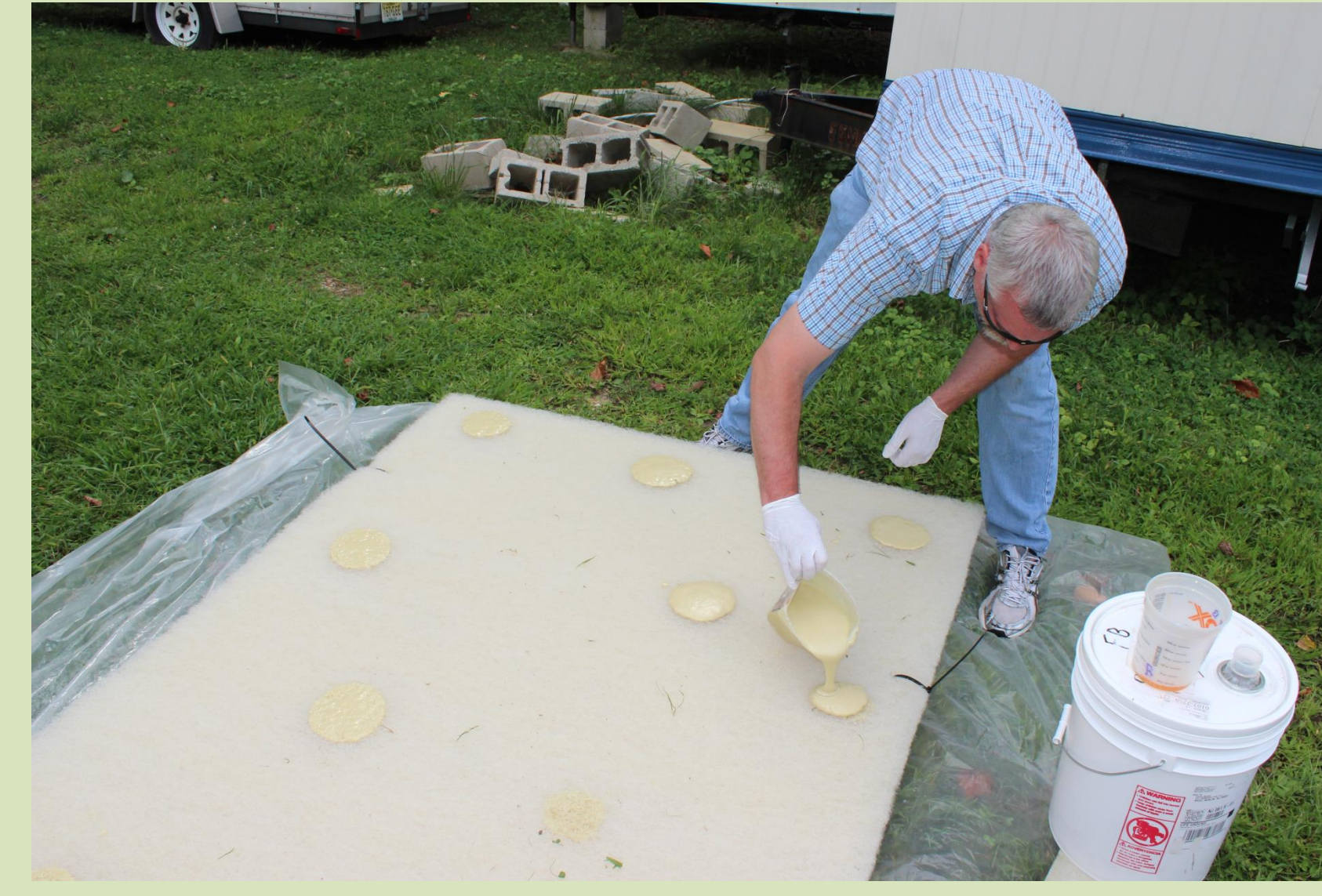
Mixing and pouring 2-part marine grade floatation material into filter material. Flows into material starting as liquid and expands into closed cell foam. Also aids to glue filter sheets together.
