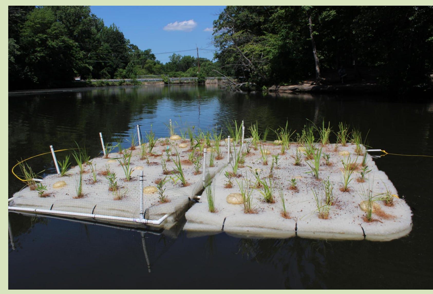
Artificial floating wetland anchored using two concrete blocks. To test for avian predation effects, 1/2 is protected with fencing and the other half is open.
