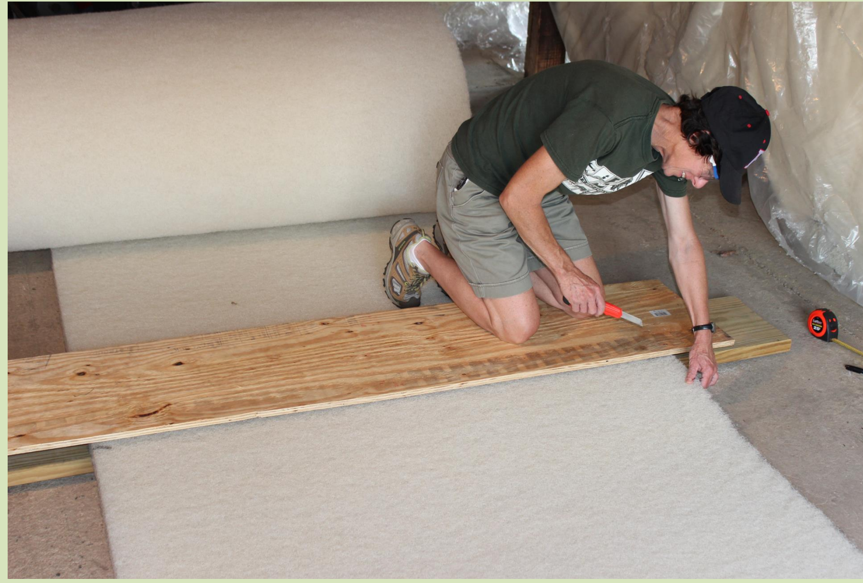
Cut three 10ft sections from a 5ft x 90ft roll of Poly-flo pond Filter material.
